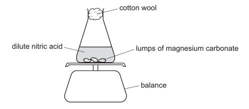
Lumps of magnesium carbonate were added to a conical flask. 40 cm³ of dilute nitric acid was then poured into the conical flask using a measuring cylinder. The magnesium carbonate was in **excess**.
