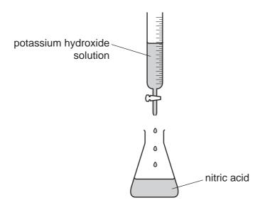
After each addition of potassium hydroxide solution the pH was measured with a pH meter and the values recorded in the table of results.
