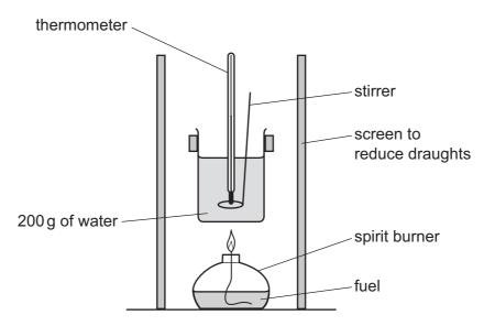
The initial temperature of the water and the temperature after heating by the fuel are recorded.
