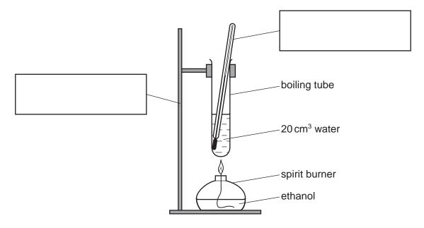
The ethanol was burned for one minute. The temperature of the water was then measured and recorded.
