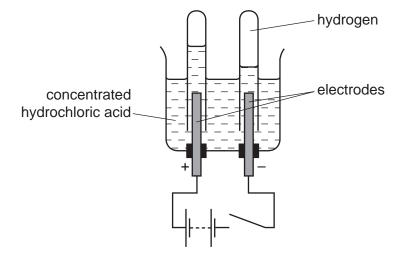
Hydrogen gas formed at the cathode (negative electrode).
