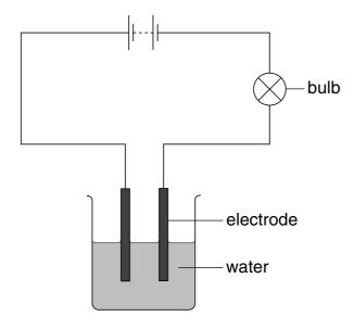
After the student adds substance  $\boldsymbol{X}$  to the water, the bulb lights.
